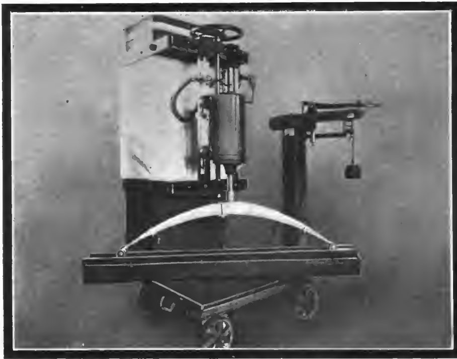
Fig. 5—Testing machine for investigating the quality and flexibility of the chassis springs, recording the deflections by means of a calibrated platform scales
